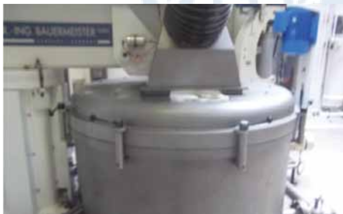
Installation of a hammer mill in place of 2-pin miller for a more efficient milling process
